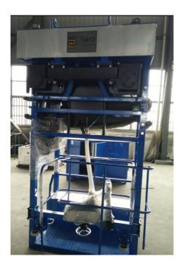
**Automatic Girth Welder** are mainly used for construction of storage tanks. Using Sub-Arc welding process, it allows faster welding time and better welding quality.
